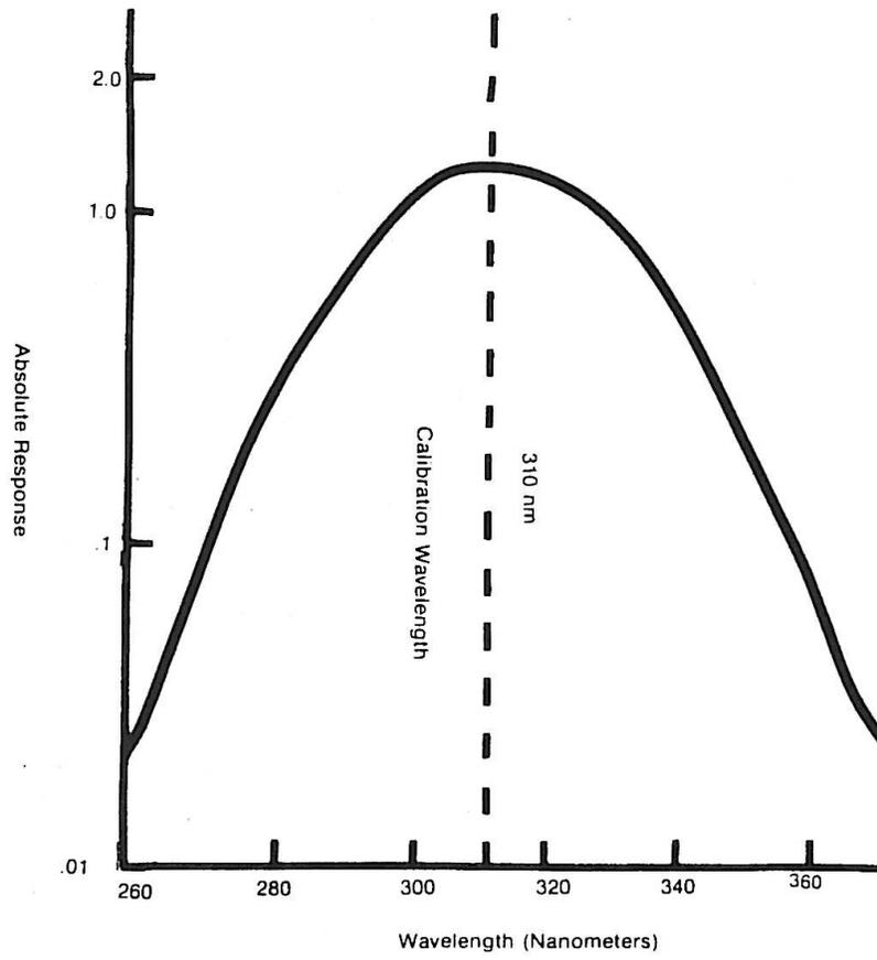
Figure 7: Typical UVX-31 Sensor Spectral Response
