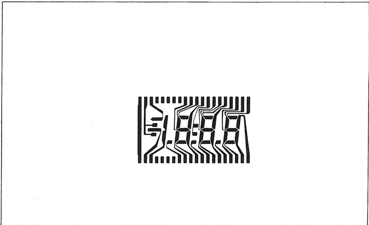
Figure 4: LCD Display Pin-outs
