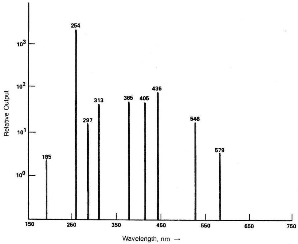
Figure 12: Typical Output From Low Pressure Mercury Lamp
