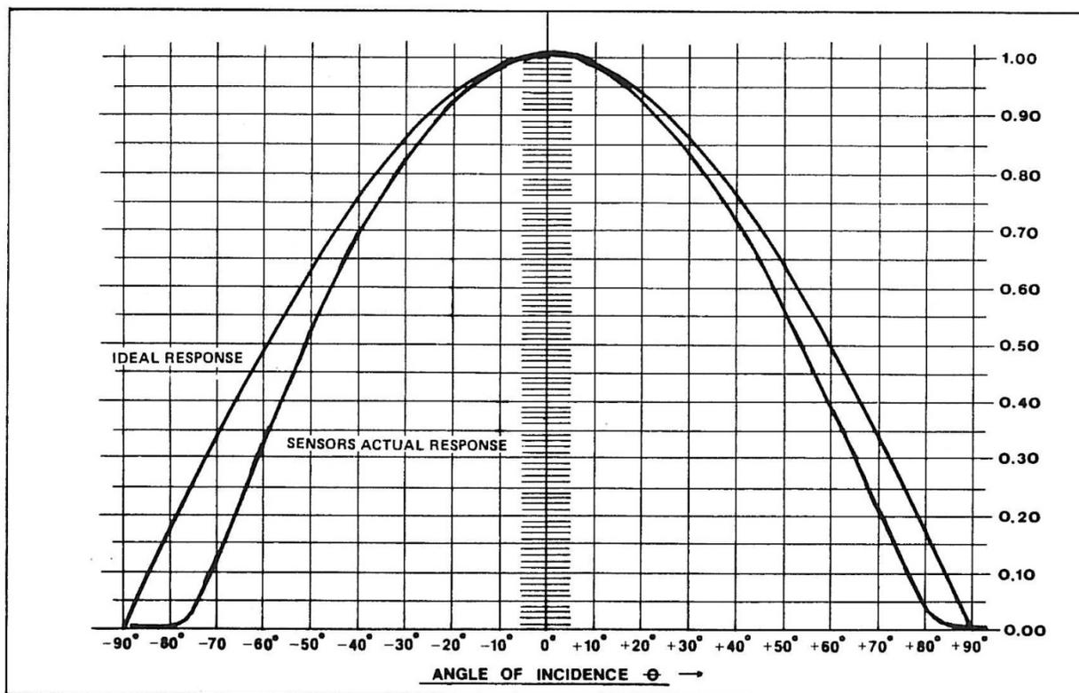
Figure 9: Typical Sensor Response Versus Incidence Angle
