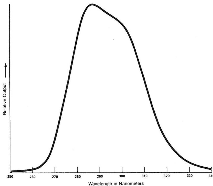
**Figure 15: Continuous Emitter, 285nm Phosphor Coated UV Lamp**
