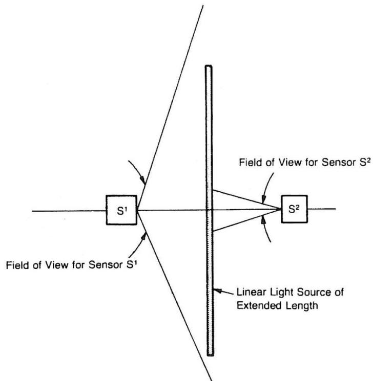
**Figure 16: Example, Illustrating Why Sensor Field of View is Important When Measuring Irradiance**
