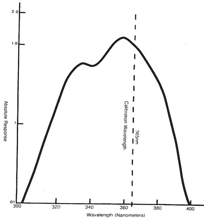
Figure 8: Typical UVX-36 Sensor Spectral Response
