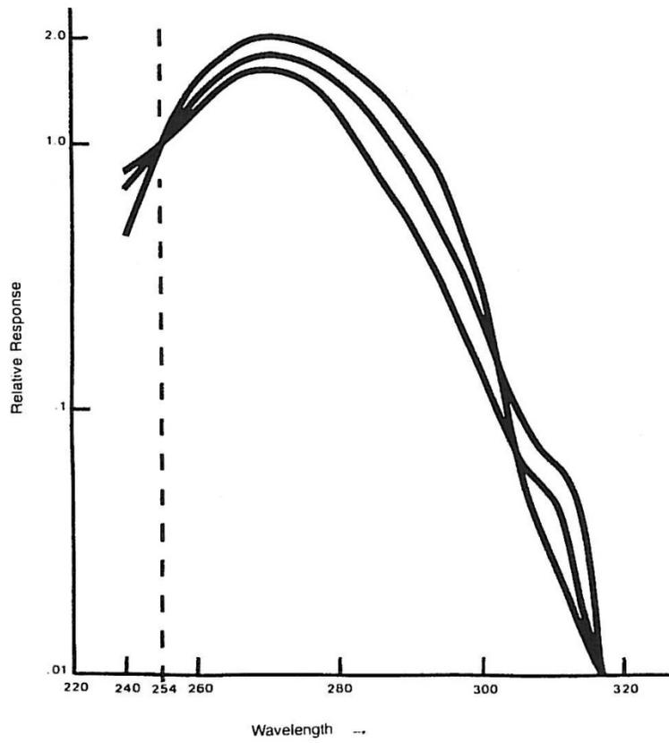
**Figure 14: Response of Three Sensors Calibrated to Yield the Same Output at 254nm Wavelength**
